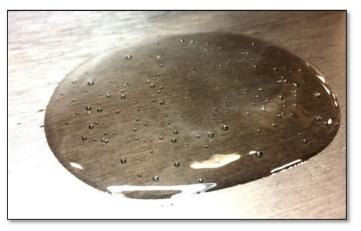
At .23% water contamination, the oil produces bubbles approximately 2 mm that quickly disappear. <u>Oil exceeds water contamination limit of .2%</u>
